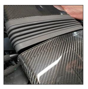
6) Bolt the snorkel to the upper boxes with the 8 provided M4 screws and metal bonded washers. Once it is attached, the engine bay should look like the one pictured below.
