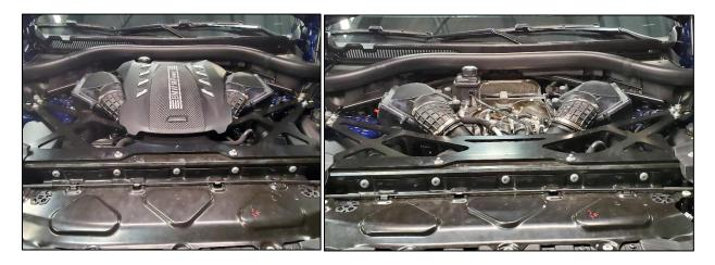
2. Remove all the push rivets and bolts holding the plastic cover, as shown. Repeat on other side as well. The sealing gasket shall be unclipped on both sides as shown below in order to properly raise the plastic cover. This operation will allow access to bolts needed in upcoming steps.
