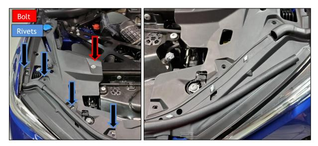
3. Remove the 12 bolts as shown below and unclip the hood latch cable from the panel. Also remove the 4 bolts holding down the front plastic panel. This will help installation of the Dinan front scoop. Remove the panel. Once out of the vehicle, remove the radiator vibration mounts. Both the bolts and radiator mounts will be re-used during the Dinan install.
