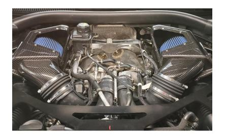
4) You can now install the Dinan Main Snorkel. Before installing, seat the main rubber boot onto the bottom of the snorkel.
