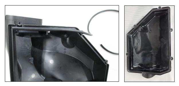
2) Install the filter into the Dinan intake lid, ensuring proper orientation as shown below. Tighten the 90-110mm clamp.
