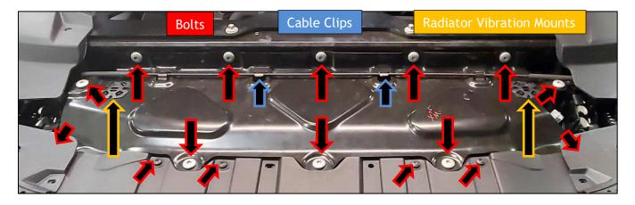
4. Once this metal plate is removed, you will have access to the air duct radiator cap. This cap will need to be modified to accept the Dinan Front Inlet.
