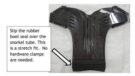
5) To install the main snorkel, slide the boot over the scoop. Make sure the boot fully surrounds the front inlet and snorkel. Check the underside fitment as an improper seal will affect performance.
