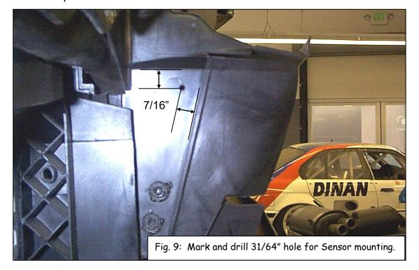
25. Mount the Sensor as shown using the 12mm nylok nut. This nut only needs to be tightened enough to hold the Sensor in place. **Don't overtighten the nut!**
