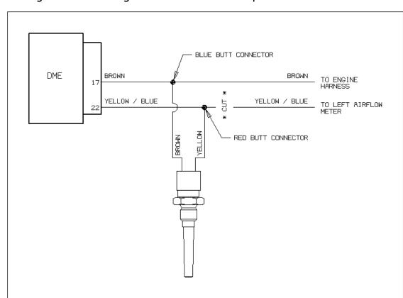
32. See Figure 11 for wiring of the Intake Air Temp Sensor.
