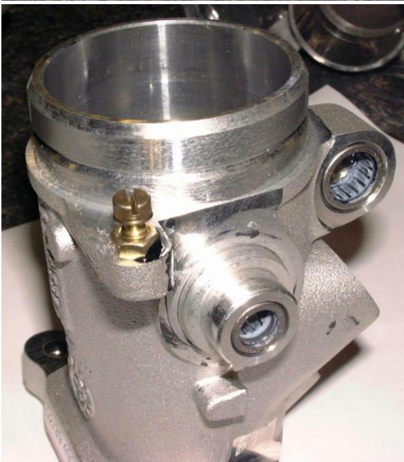
Cyl # 3 This one has the bearing in the throttle shaft hole.
