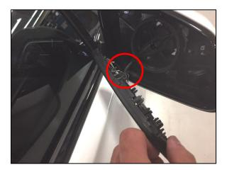
5. Locate the 2 tabs on the inside of the mirror housing. Use a small screw driver and/or a pick to release the tabs. As you have one of the tabs released, pull on the mirror cap unit to pop it lose. Repeat this on the other side.
