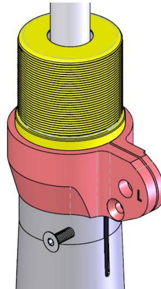
12. Install the spring perch and black plastic isolator disc (in Coil-Over Hardware Kit) as shown. Adjust the perch to its lowest setting. This will be the starting ride height setting, and should get you very close to Dinan's target bumpstop clearance. Snug the 6mm screw to lock the perch into place.
