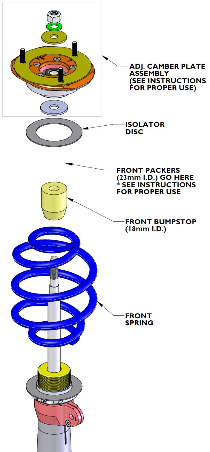
14. Install strut assemblies into vehicle, taking care to align the slots left-right to allow camber adjustment. If there are circlips on the camber plate studs, they may be left in place as they keep the assembly together while you install the struts into the car. These clips will not interfere with your ability to adjust camber.
