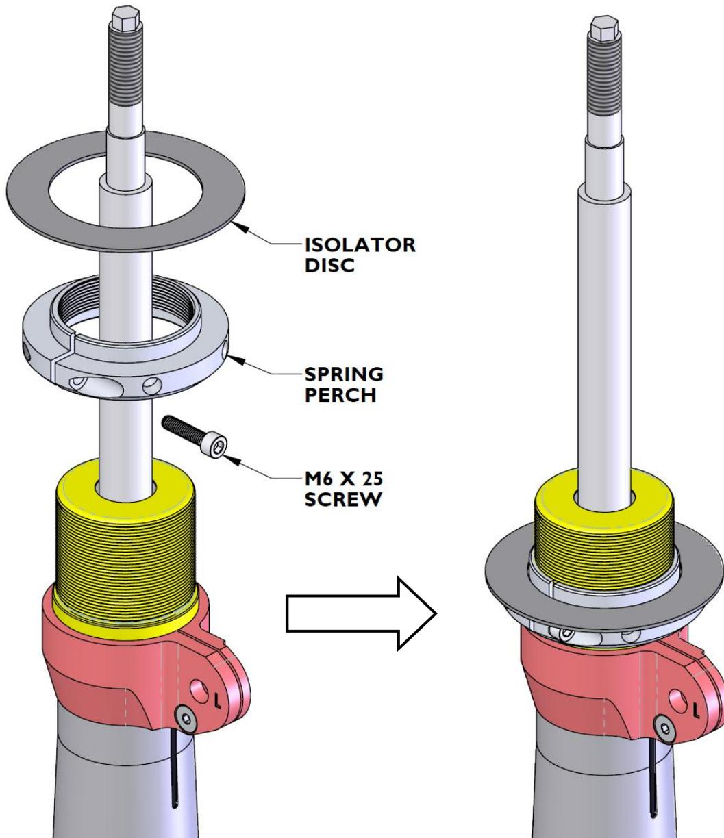
13. Install the rest of the front strut components as shown. Please note:
