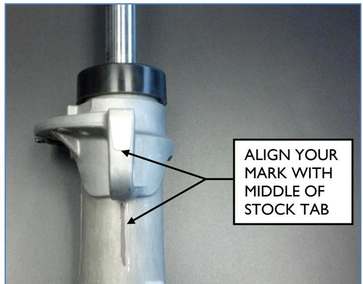
4. Once the tab locations have been marked, remove the plastic caps from the top of the struts. These will not be reused.
