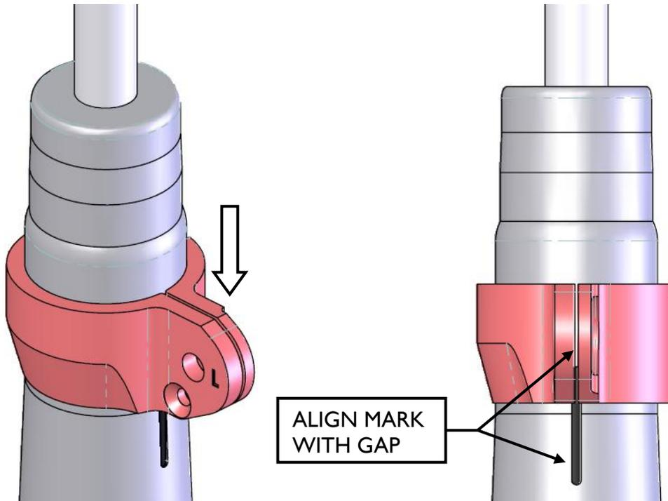
8. Locate the two Front Threaded Perch Assemblies. These are the same for left & right. Verify that the O-rings are properly located in the grooves as shown in figure.
